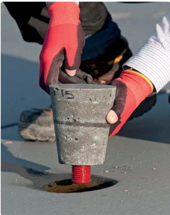
Lifting hole plug cast in C-Defence high-abrasion-resistant concrete formula showing cast-in nylon thread.
